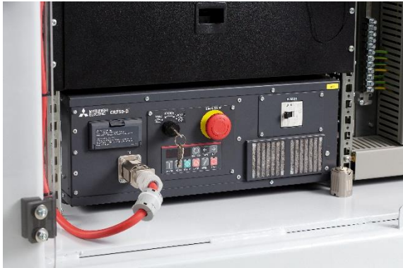
Image 3: The overall size of the robot cell is just 4 m 2 , which is made possible by the compact dimensions of Mitsubishi Electric's CR750-D robot controller.
