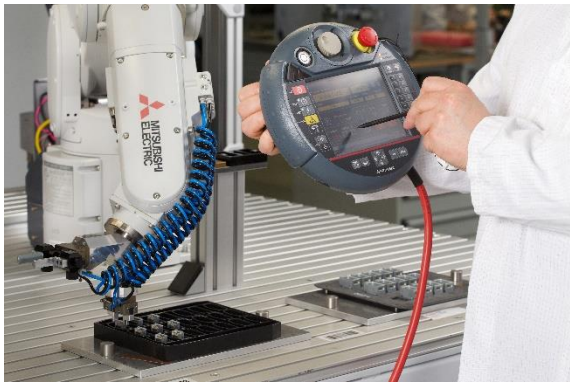
Image 4: The user can intuitively program the Mitsubishi Electric robot in a matter of minutes using the teaching box.
